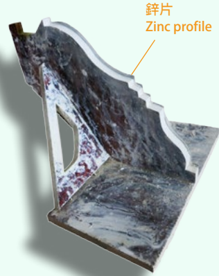
◀ 這個模板上裝有鋅片，鋅片的邊緣切成仔細坑紋，與未受損的簷口坑紋相同。運行於最終面層的石膏時，這模板讓技師劃出準確精工簷口裝飾線。 A 'horse' with zinc profile for 'running' cornices. The zinc profile for running the final finishing plaster layer is carefully cut to match the required cornice profile.
